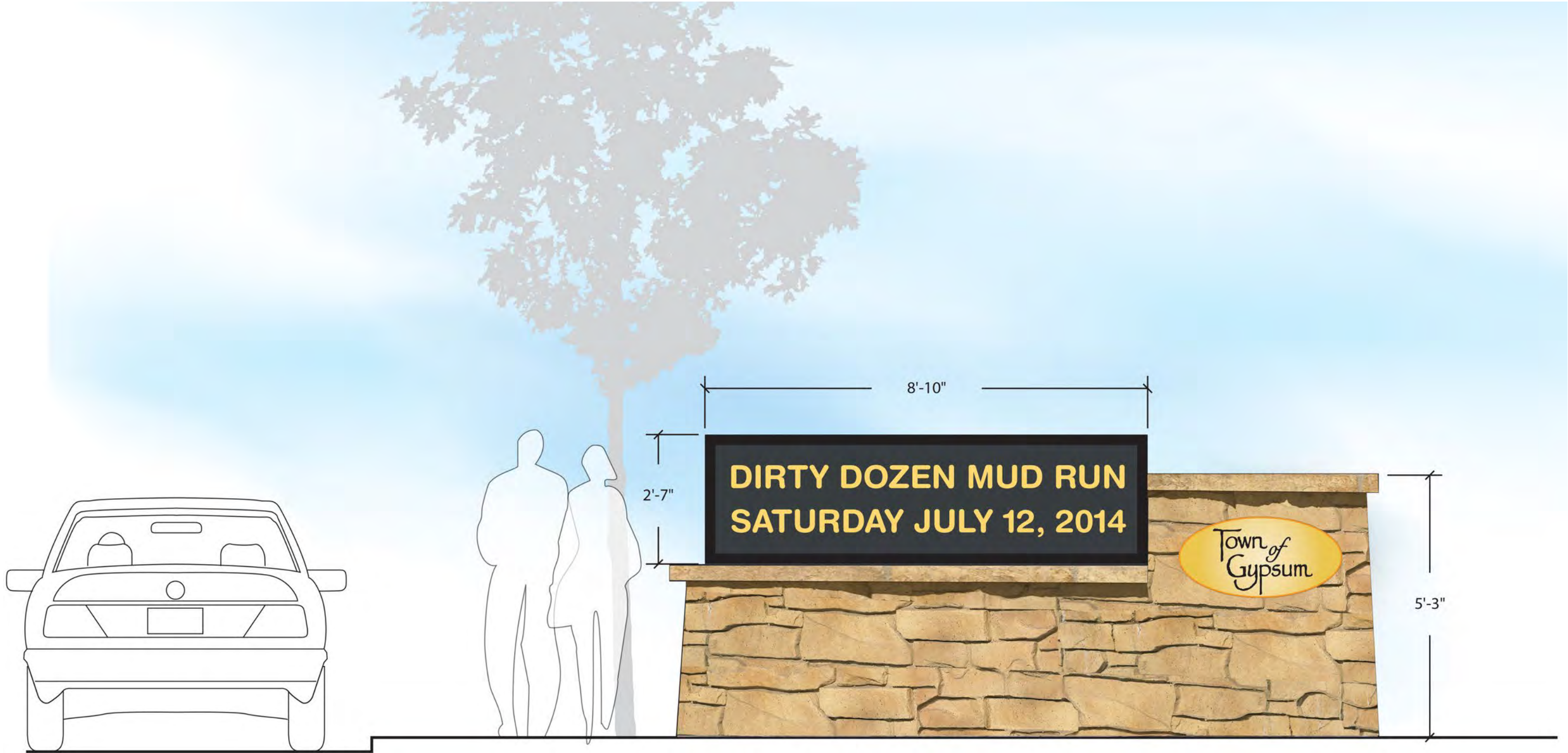
Gypsum Variable Message Sign: Option 2 (Stone wall base) LED, text only, non-animated Scale: 1/2" = 1'-0"
